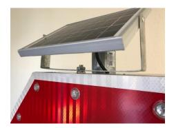
2. Connect Solar Panel to Stop sign by connecting Mail End of black cord to Female end and screwing together with your fingers until female end is screwed on tightly. For extra weather proofing, it is recommended to use black electrical tape and tape over connection completely by going around the combined male and female parts.
